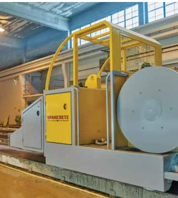
The Spancrete Multi-Function Machine carries out different tasks, from cleaning the top surface of the casting bed and collecting waste, to pulling the strands on a clean casting bed, as well as oiling the bed just prior to production. It features 4-wheel drive for easy operation and the flexibility of pulling multiple strands in one pass for the full length of the bed, providing the ultimate in efficiency.
