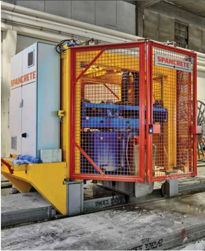
Spancrete Saws are used to cut the hollowcore to the desired length after the concrete is cured. Certain saw models are capable of sawing angles from 0-180 degrees. The Saws are fully adjustable to perform well in each specific environment.
